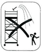
working plat-form. Only re-lease the load when the recipient of the load is s ecure in hands.
